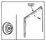
Caution: This access panel covers a 2" NPT plug that was required during the manufacturing of this water heater. This 2" NPT flange is not a cleanout fitting, removing the 2" NPT plug and using this fitting as a cleanout could void your warranty.
